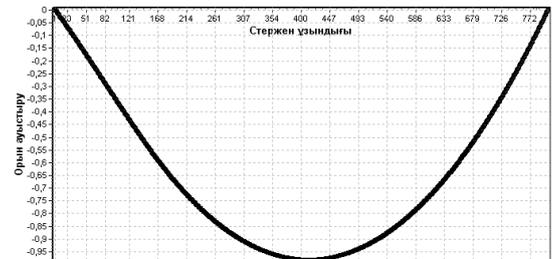
Figure-3 - The law of distribution of displacements of nodal points along the length of the rod with  $q = -70(W/cm^2)$
