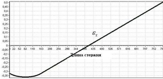
Figure-4 - The distribution field  $\varepsilon_x$  along the length of the rod with  $q = -70(W/cm^2)$
