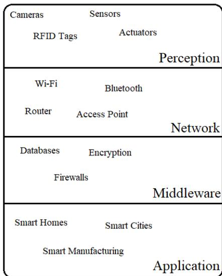
Figure 1: The four architectural layers of IoT
