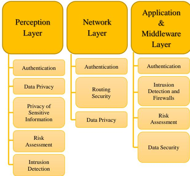
Figure 2: Countermeasures proposed for the four architectural layers of IoT
