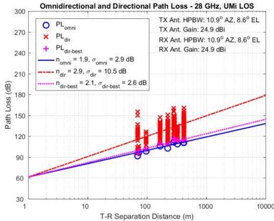
Figure (6) Path loss for 28GHz band (LOS)
