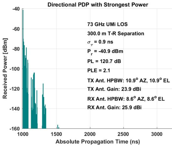
Fig. (2) Directional PDP for 32X4 LOS 73GHz
