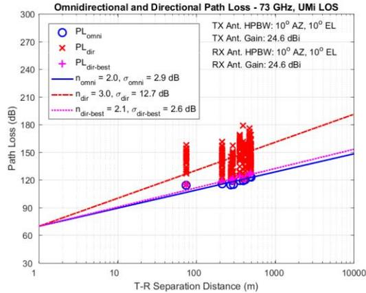
Figure (7) Path loss for 73GHz (LOS)
