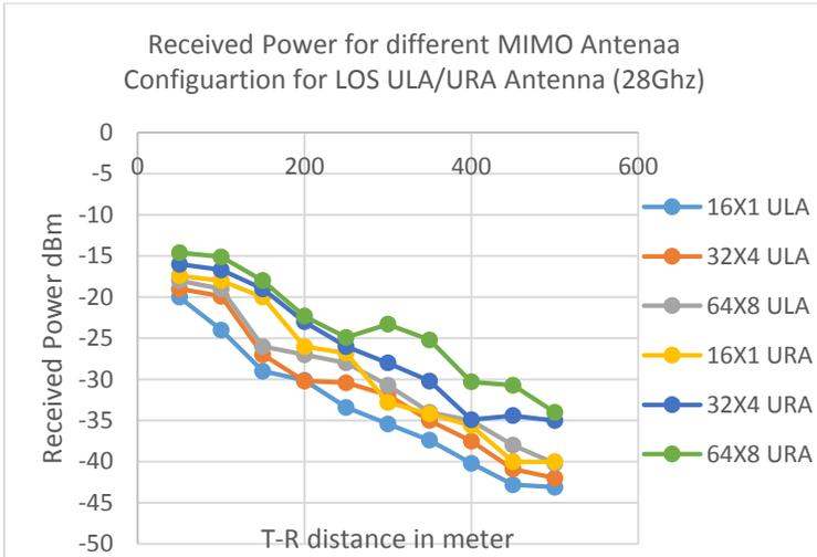
Figure (9) The received power using two types of antenna (ULA and URL)
