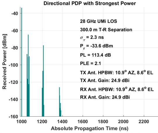
Fig. (1) Directional PDP for 32X4 LOS 28GHz
