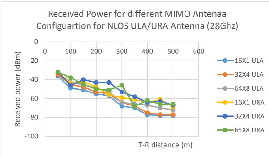
Figure (11) The received power using NLOS ULA /URA antenna
