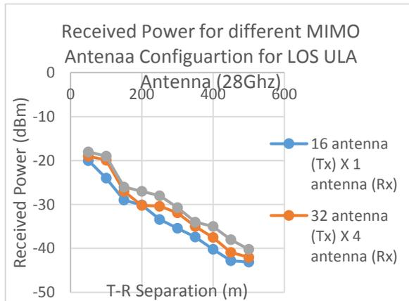
Figure (8) Effect of increasing number of antenna at Tx and Rx
