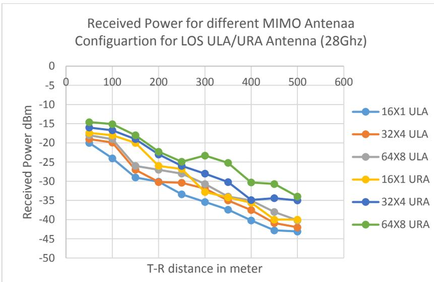
Figure (10) The received power using LOS ULA/URA antenna
